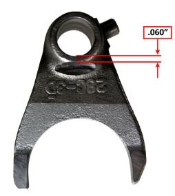
To check clearance, place primary shaft and fifth gear in place
